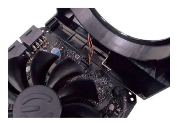
11) Place one thermal pad on the back of PCB.
