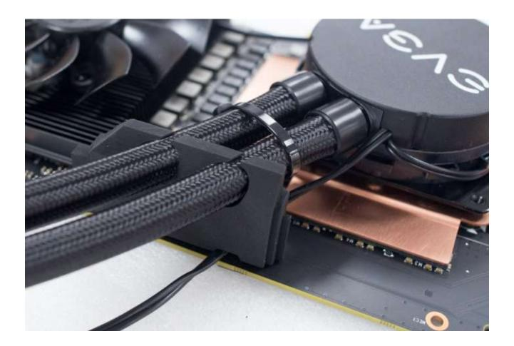
10) Plug in the 2-pin LED power cable from the shroud into the LED header. Use the picture below as a guide:
