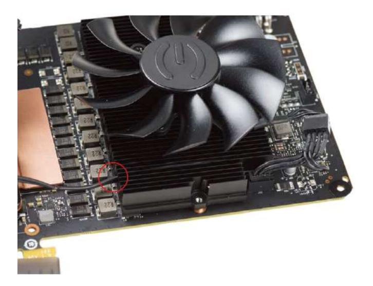
9) Attach the included rubber insert to the edge of the card, which will be used to hold the tubes in place. Make sure to run the fan-connector underneath the small channel provided under the rubber insert.
