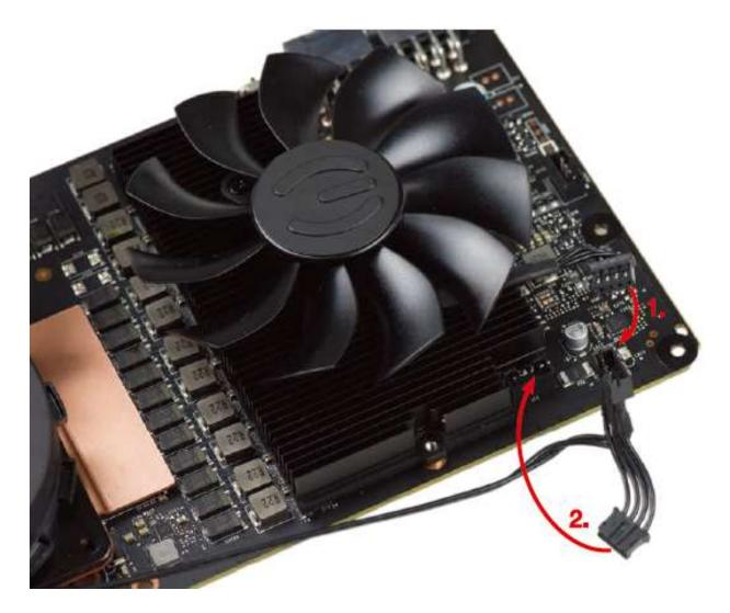
8) Use the fins in the heatsink to run the wires underneath the fan, then gently flatten the cables parallel to the PCB. We recommend using the 6<sup>th</sup> fin from the bottom, as shown in the pic below.
